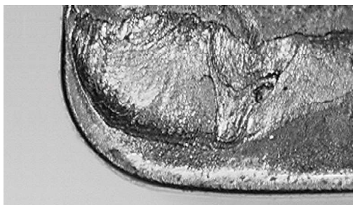
The hot chip which is being evacuated causes cratering at the rake face of the cutting edge.
